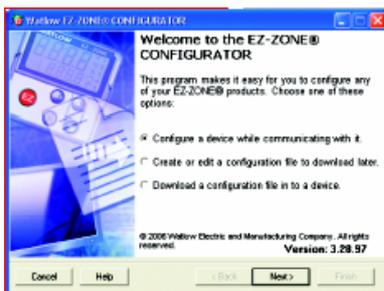
The EZ-ZONE Configuration software allows WATLOW controllers to be configured in one simple process via your PC. The software uses standard bus communications protocol that is included with all EZ-ZONE products.
